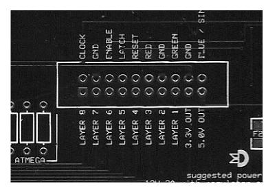
LAYER X – Active LOW inputs to select which layer is active. These are usually only active one at a time and cycled quickly to give the illusion that they are all on when viewing the cube. Although you CAN write your code allowing more than 1 layer to be active at once, it is not recommended as this will cause a current increase that may blow the fuse on the 5V line.
