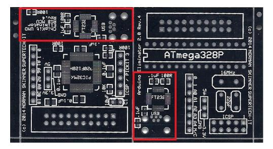
For the newer separate snap apart eliminators that you may have ordered in addition to your V4 or higher boards, please do not install any of the components in the red area. Because of a problem with the FTDI chips, this function is not implemented. Also please note you MUST use the non-SPI layer code, as the additional shift register has been removed from the Arduino eliminator.
